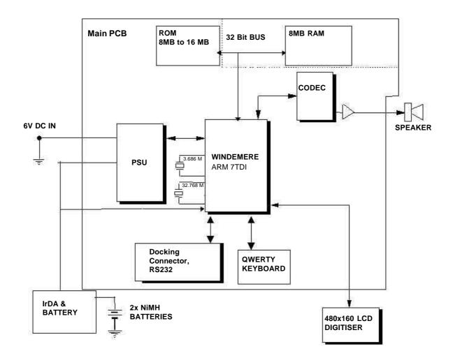
The Revo electronics are contained on one main PCB with the IrDA and Battery interface on a second small PCB in the Battery compartment of the product. By having a separate compartment for the battery, any heat generated by the main PCB does not affect the temperature sensing on the battery pack
