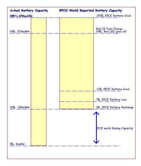
Revo uses a "Gas Gauge" chip to measure the charge put into, and taken out of, the internal NiMH battery pack. From this Gas Gauge a battery charge capacity is calculated and shown to the User. The User will only ever be able to use between 30 and 100% of the Battery's real capacity which allows the machine to preserve data for upto two weeks. Note that this is shown as a capacity of 0% to 100%.
