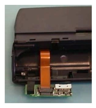
To remove the lower spine moulding first remove the battery and IrDA/Power PCB then gently flex one of the side walls of the lower spine moulding.
