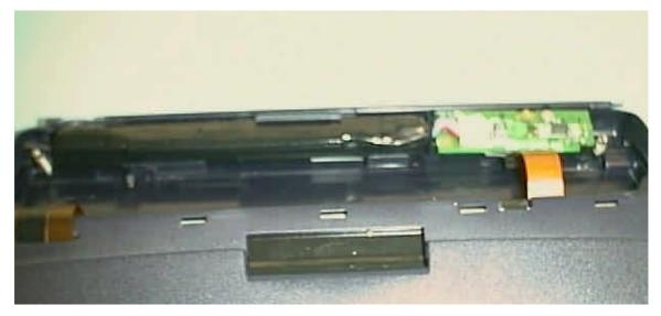
To remove the battery first pull away the tape covering the battery clip, then disconnect the battery from the IrDA/Power PCB, take care not to damage the plug or socket. The battery is clipped in place and can be pulled out of the lower spine moulding.
