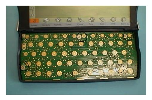
Using the LCD/PCB Extractor (see Photo) gently lift the rear edge of the PCB upwards and hold it in place, take care not to damage the two Flexi cables attached to the PCB, now lever the front edge of the PCB backwards, the PCB will hinge and lie flat against the LCD. Take care not to damage the PCB or LCD during this operation.
