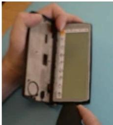
To fit a new LCD first feed the flexi cable through the slots in the upper and lower moulding. NOTE, you will have to remove the outer logo label and the hinge pins from the spine moulding to insert the Flexi cable of the new LCD module. Once the Flexi is in place the LCD simply clips into position.
