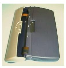
Unclip the two hinge springs from the upper spine moulding, you should take care not to damage these springs as they are heat staked to the lower spine and if damaged the entire moulding must be replaced.
